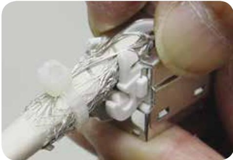
10. Push the shield cover into place, securing the shield cap to the completed assembly.
