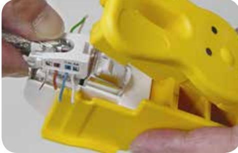
5. Place the assembled adapter body and cap into the Termination tool supplied with the adapter.
