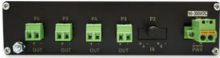
Figure 2 – Rear panel of ITD, configured with four TTL outputs
