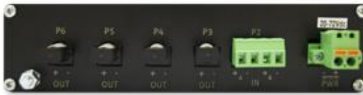
Figure 3 – Rear panel of ITD, configured with four fiber outputs
